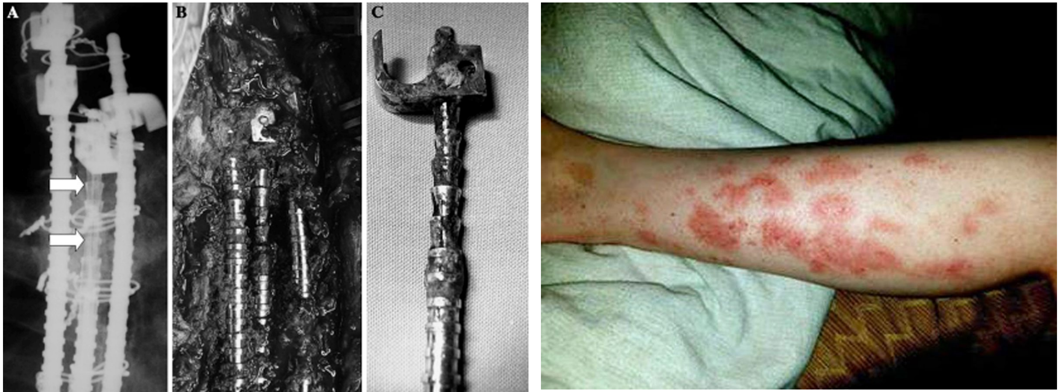
Radiological signs of corrosion in the proximal end of the rod (a) (arrows). Macroscopic corrosion of the implant was evident during surgery (b) and in the examination of the retrieved instrumentation (c)
